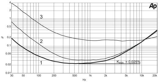
Curve 1: Bias adjusted correctly; bias high with selected tubes
