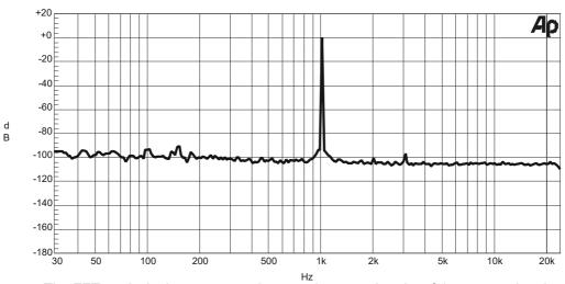
The FFT analysis demonstrates the superb spectral purity of the output signal. No mains-borne noise (normally at 50 and 100Hz) is present
