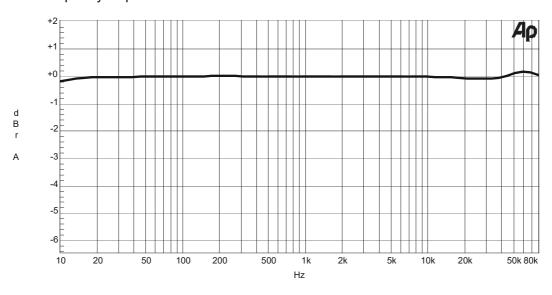
Between 10 Hz and 90 kHz the frequency response tolerance is within 0.3dB  $\pm$
