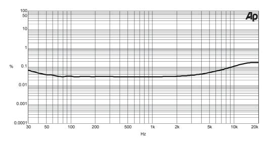
The total harmonic distortion curve is very linear, increasing only slightly at the lowest frequencies. This performance is only possible using a highly specialist output transformer.
