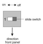
Rippled records can create subsonic disturbances. The subsonicfilter eliminates this disturbances. Cutoff frequency is 15 Hz
