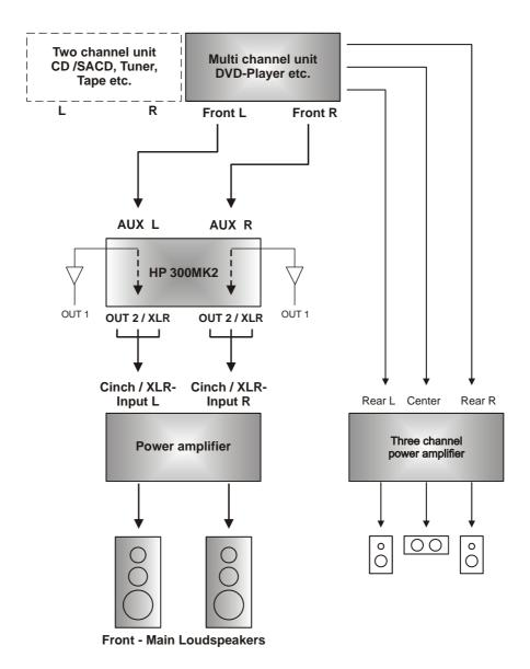
In the multi channel mode the common volume of the multi channel system has to be adjusted at the multi channel source, eg the DVD player, TV, etc. In the bypass mode the volume control of the HP 300 MK2 is out of function except the output 1.
