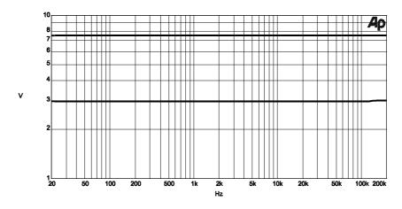
Frequency response accuracy of line stages in 'low gain' setting. 20 Hz - 200 kHz: 0.1 dB
