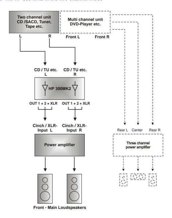
In the two channel mode all three outputs are regulated and amplified. In the two channel mode the AUX input can be used as a normal line high level input
